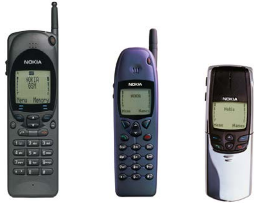
Figure 6. The evolution of Allgon’s terminal antenna designs: a) is a extractable \lambda/4 wave antenna with a bottom helix, b) is a short helix and c) is an inbuilt PIFA (Planar Inverted F Antenna), not seen.
