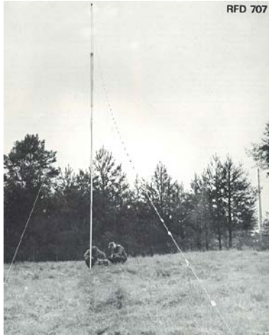
Figure 4. The reflection free directional broadband antenna RFD707. The reflection free directional broadband antenna RFD707, was a lightweight HF antenna for military field operations. Similar products are still in use by armies all over the world today. Since it was a thin wire antenna, it was internally at Allgon referred to as the “Hallén- antenna”(referring to the great Swedish antenna professor [3]).
