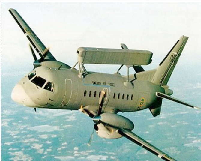
Figure 6. The ERIEYE radar mounted on a Saab 340 turboprop aircraft.
