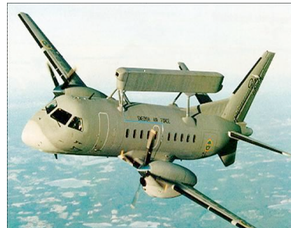
Figure 14. The ERIEYE radar mounted on a Saab 340 turboprop aircraft.
