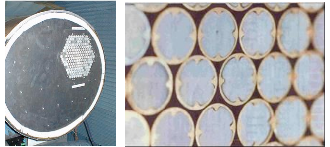
Figure 18. (left) AESA testbed, (right) dual polarized dielectric loaded radiating elements.
