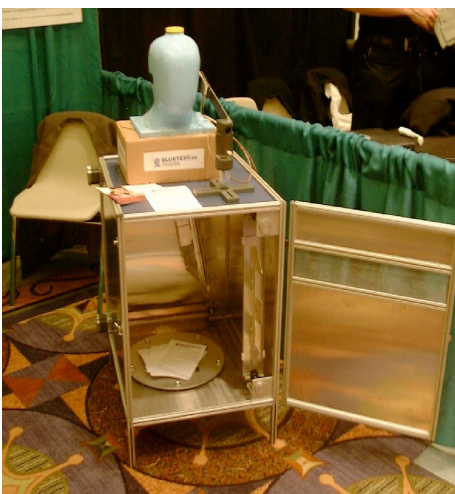
Figure 9. Early prototype chamber for Bluetooth measurements showcased at the IEEE International Symposium on Antennas in 2000.
